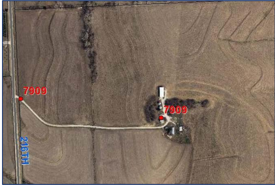
Figure 2. Placement of address point on primary entrance path within a parcel boundary as shown on the left address point for 7909. The illustration also shows the placement of the address point on the primary structure footprint. This is helpful in cases where the primary building is difficult to see from the primary entrance path off an addressed road.
