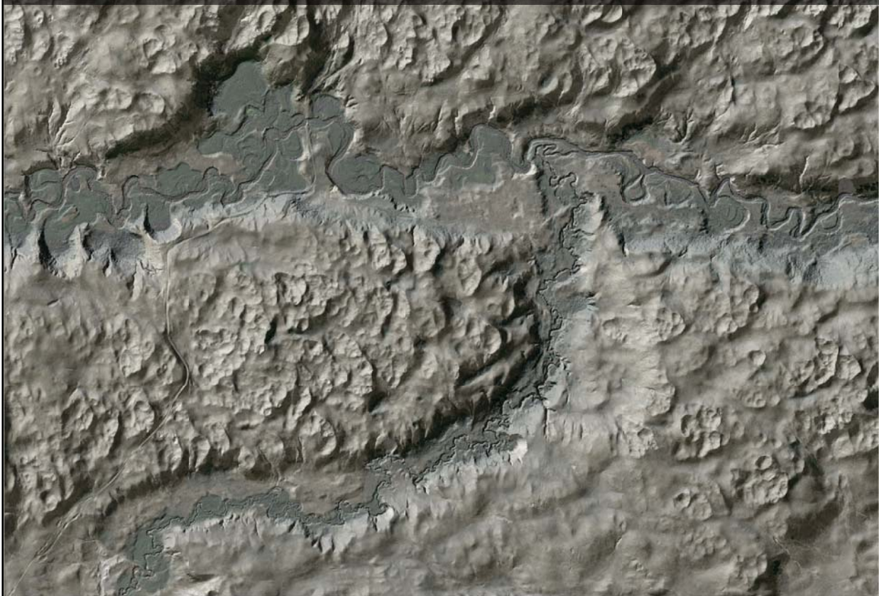
2014 NAIP image draped on hillshade of LiDAR derived digital elevation model.
